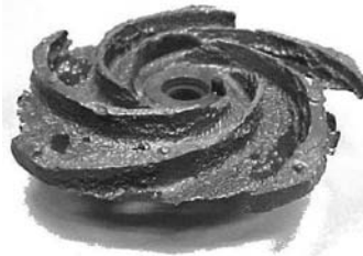
Fig 7 Worn impeller from condensate pump
